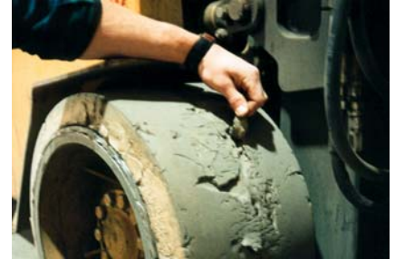
Deteriorated Floors Drain Productivity from Operations and Increase Material Handling Vehicle Maintenance Costs
